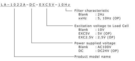
Modification of Power supplied voltage, Excitation voltage and Filter characteristics is optional (OP) at the factory.
